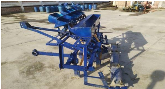
Improved seed meters for seeding both large and small grain seeds (2021-22)
